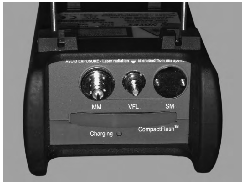
FIGURE 33.42 The VFL is built into this OTDR.
