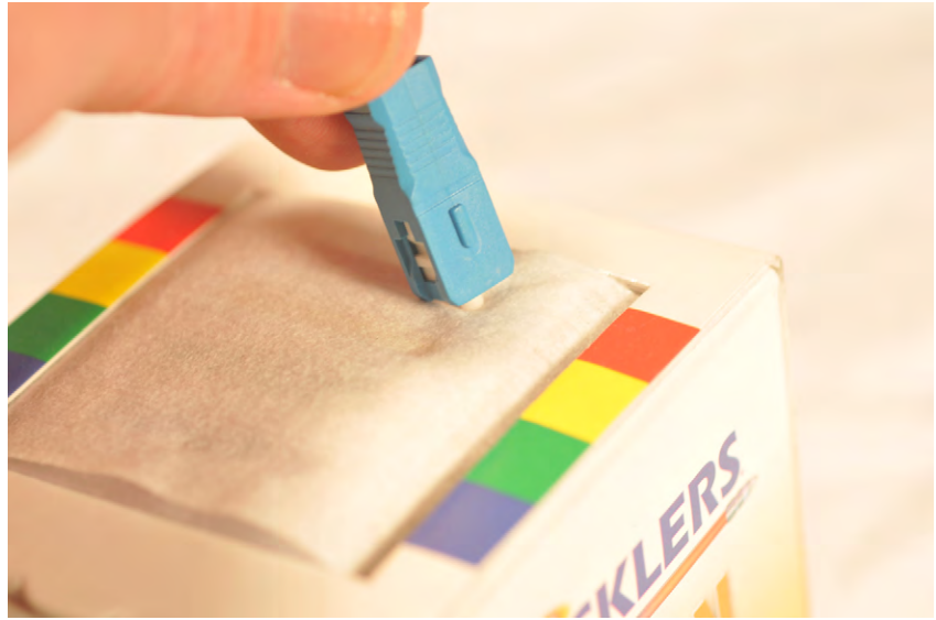
FIGURE 26.89 Connector properly placed in the slot for cleaning the endface
