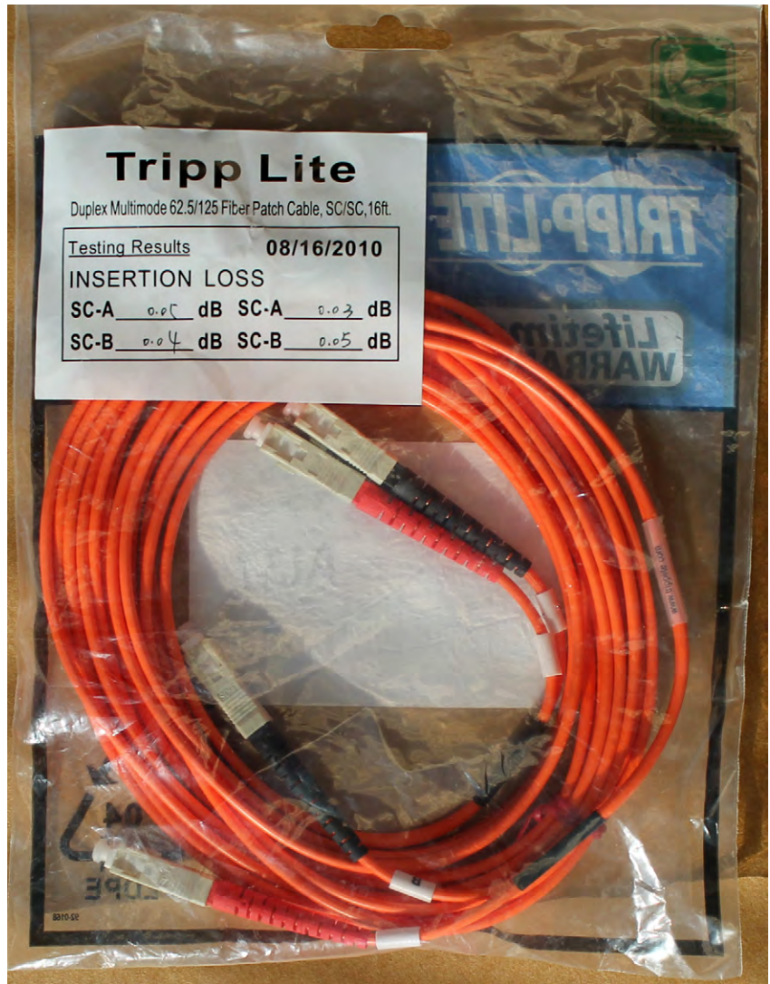
FIGURE 33.37 Duplex multimode fiber patch cable with connector insertion loss measurements on the packaging
