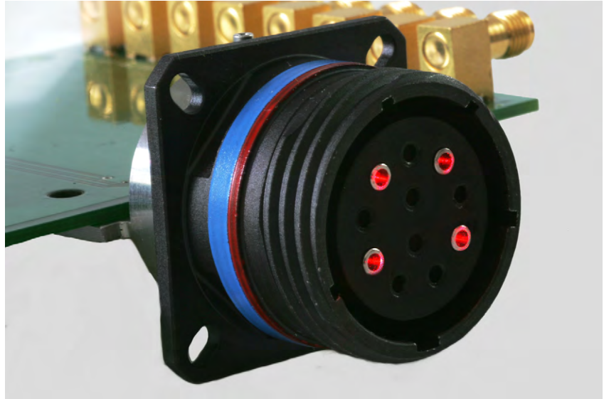
FIGURE 28.18 Transceiver bulk-head receptacle soldered to the circuit board
