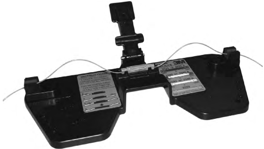
FIGURE 25.37 Mechanical splice tool properly set up to perform a mechanical splice
