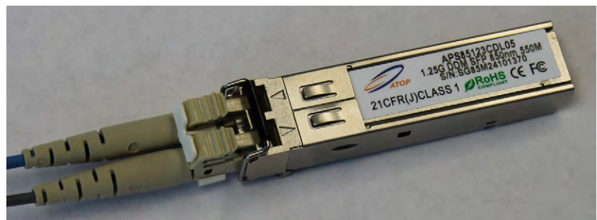
FIGURE 30.4 850nm 1.25Gbps transceiver with an LC transmit and a receive receptacle
