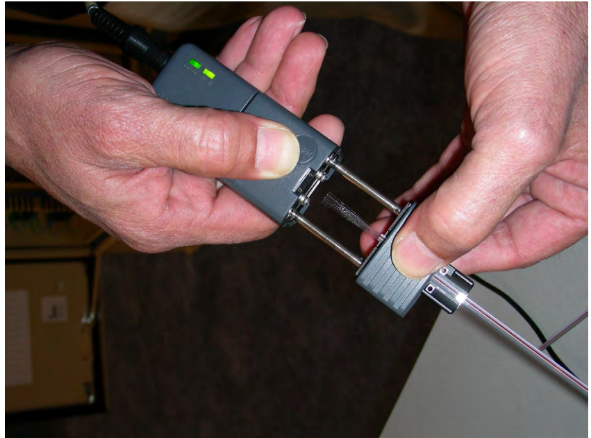
FIGURE 25.42 Ribbon fiber stripper using heat to remove the Mylar tape and coating
