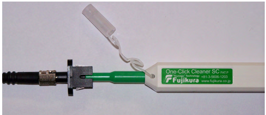
FIGURE 34.24 Cleaner tip inserted in ST-to-SC adapter
