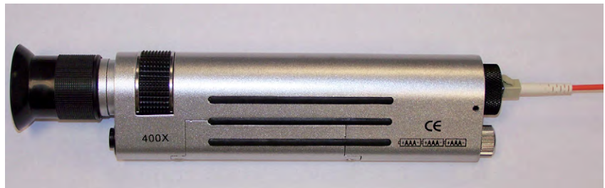
FIGURE 26.100 400X microscope with an LED for illumination and an LC connec- tor inserted for inspection
