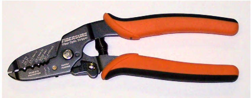
FIGURE 26.51 Stripper designed to remove the jacket, tight buffer, and coating
