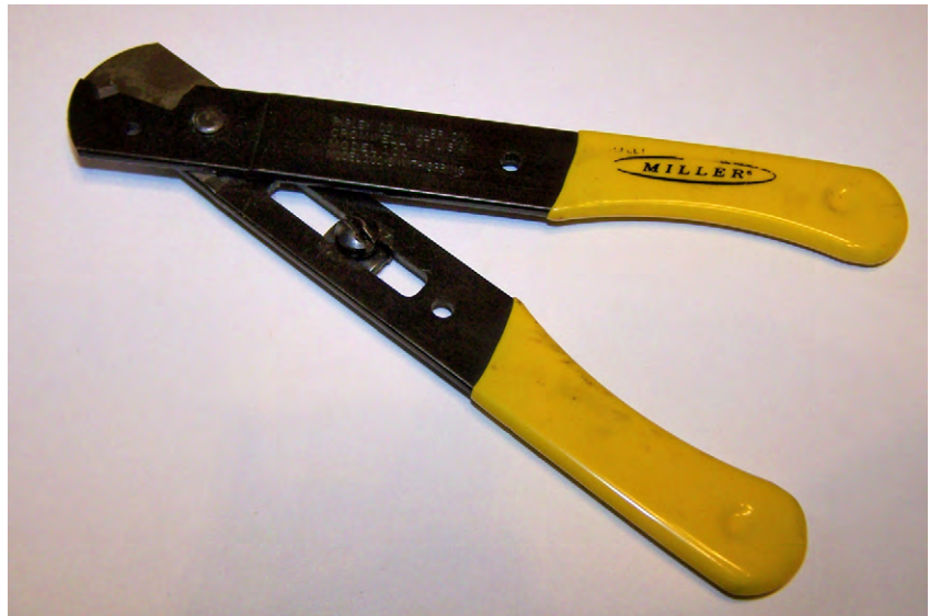
FIGURE 26.52 Adjustable stripper that can be set to remove the jacket, tight buffer, or coating
