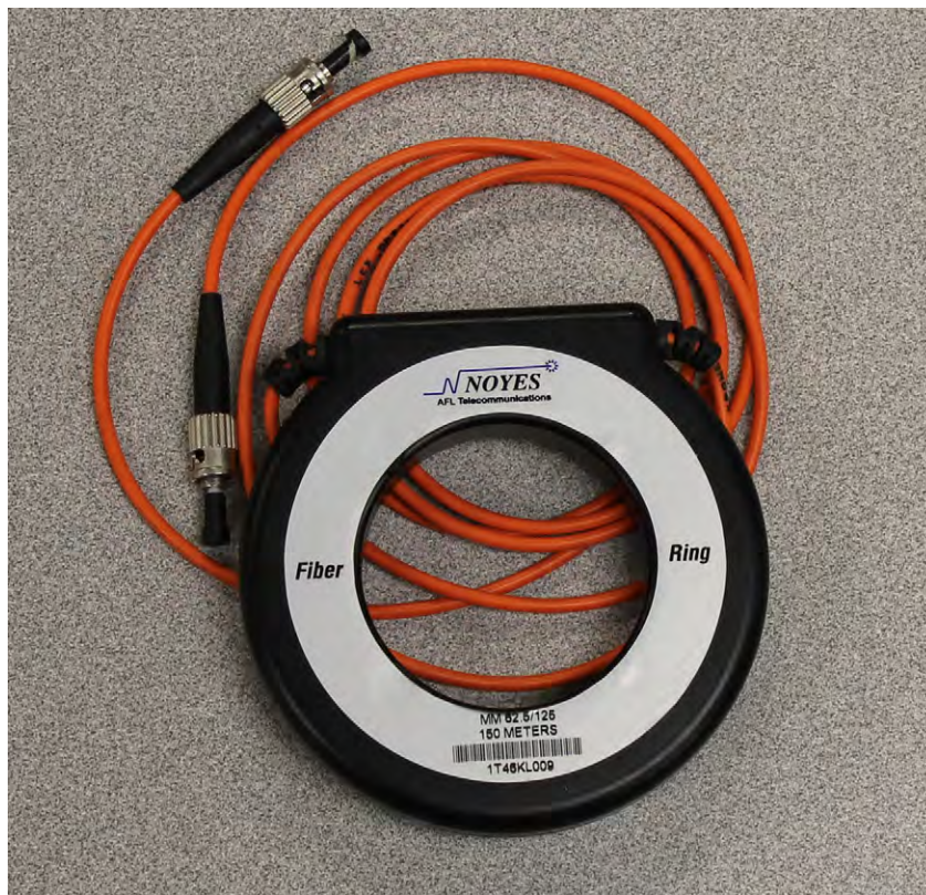
FIGURE 33.50 Compact ring-type launch/receive cable
