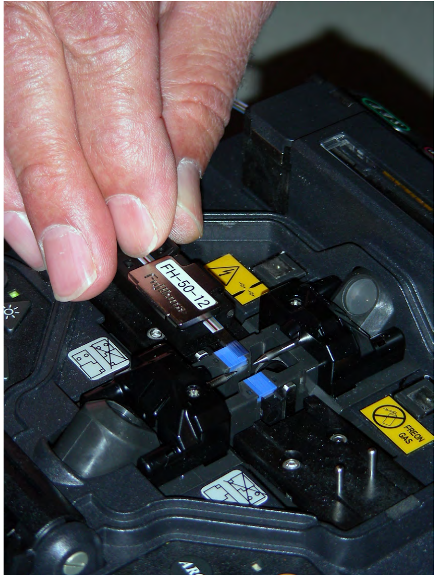
FIGURE 25.45 Ribbon fiber placed in the fusion splicer for splicing
