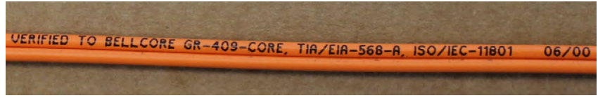
FIGURE 24.31 Duplex cordage manufactured in June 2000
