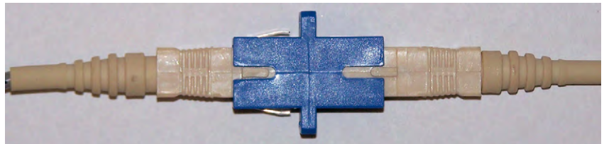
FIGURE 34.14 SC-to-SC mating with connector on right not fully mated
