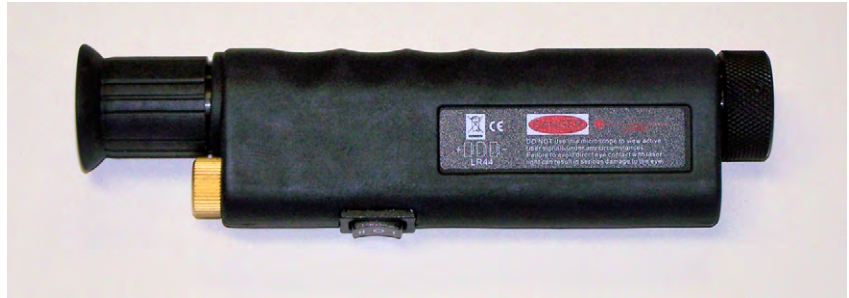
FIGURE 26.99 400X microscope with a laser for illumination
