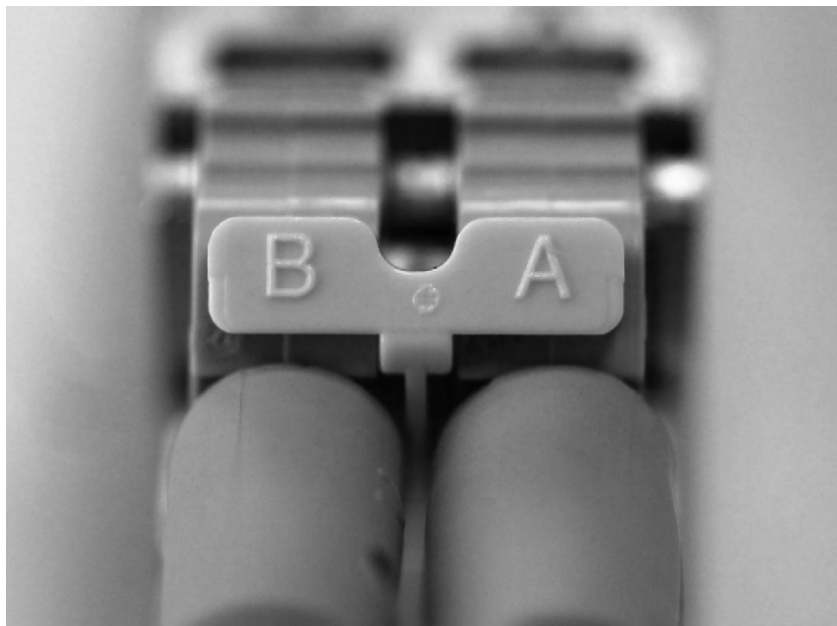
FIGURE 31.27 A raised letter latch holding two LC connectors together
