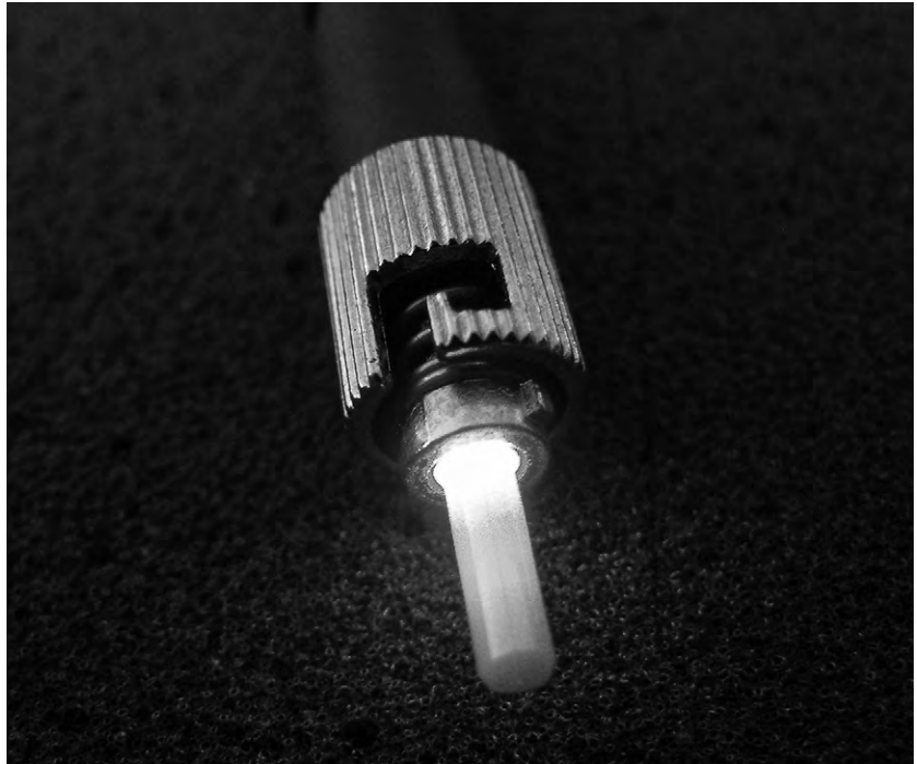
FIGURE 34.35 Broken optical fiber in ST connector ferrule being tested with VFL
