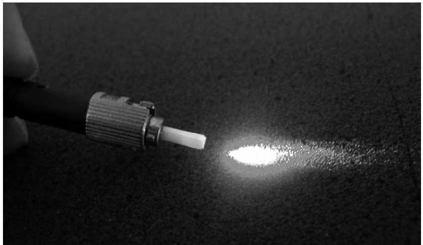
FIGURE 34.36 Good ST connec- tor being tested with VFL
