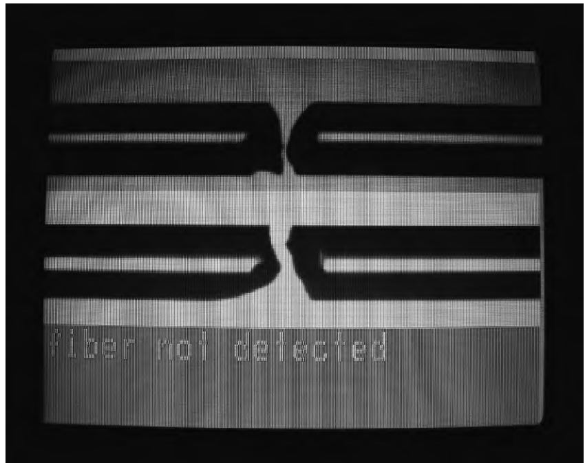
FIGURE 25.32 Optical fibers with jagged endfaces viewed on the display of a fusion splicer
